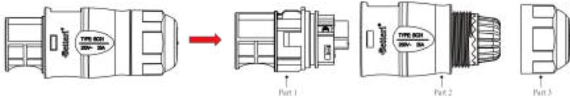
2. Insert the AC cable from Part 3 to Part 2, and complete the wiring for the L, N and Ground inside Part 1 AC Port accordingly:
