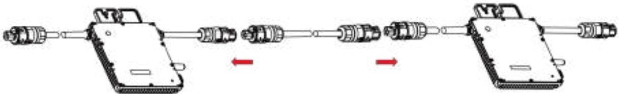
B) Install the AC end cap on the open AC connector of the last microinverter in the AC branch circuit.
