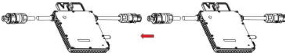
*\*Note: The length of AC cable on microinverter is around 1.23m. If the distance between two microinverters is more than 1.21m, please use the AC extension cable between two inverters (As picture indicated below).*
