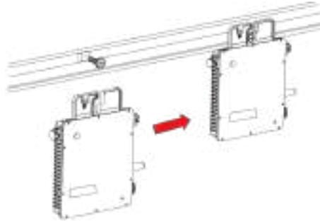
*\*Note: Please install the microinverter at least 50cm above the ground/roof for better communication with Hoymiles DTU.*
