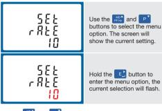
Use the property and p buttons to choose the desired pulse rate. To save the new setting, hold the button for 3 seconds until the selection stops flashing
