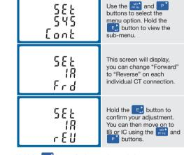
Hold the WA button for 3 seconds to exit the set up menu.
