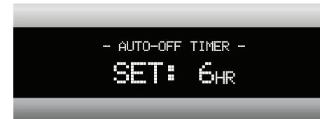
The Auto-Off Timer is used to specify a specific charging time (2, 4, 6, 8, 10 hours), after which the InLine® USB Smart Control Multimeter stops the charging process automatically. To set the Auto-Off Timer, press and hold the button until the corresponding display appears. Release the button briefly, then press it again.
