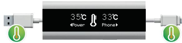
The InLine® USB Smart Control Multimeter has temperature sensors on both ends of the cable to check your power source and your mobile device, as shown by an indication of the measured temperature on the display. Charging is terminated as soon as elevated temperatures are detected (from 55°C when charging with less than 7.5W / from 65°C when charging with more than 7.5W).
