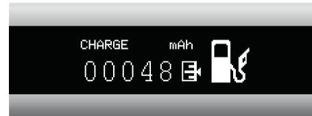
To measure the mAh capacity of a powerbank, the powerbank should be discharged before starting the measurement. Charge the powerbank by connecting it to the InLine® USB Smart Control Multimeter and the InLine® USB Smart Control Multimeter itself please connect to an USB power source. As soon as the charging process is completed, the last mAh value shows the capacity of the charged powerbank. Use the same procedure to measure the battery capacities of smartphones and tablets.
