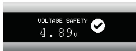
The microprocessor of the InLine® USB Smart Control Multimeter monitors the voltage from the power supply to the receiver for signs of failures or overloads. This is especially critical when using third-party USB power supplies. The InLine® USB Smart Control Multimeter stops charging process if voltages (< 4.5V) occur.
