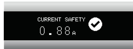
The microprocessor of the InLine® USB Smart Control Multimeter continuously monitors the current flow from the power supply to the receiver. When there is a strong increase in current flow (> 2.5A) the InLine® USB Smart Control Multimeter stops charging automatically.
