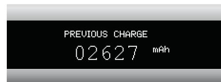
The „Previous Charge“ display shows the last charged capacity. It is quite common for users to leave their InLine® USB Smart Control Multimeter connected when smartphone or tablet is fully charged. Keep in mind that these devices continue to consume energy when they realize that the battery capacity decreases again, for example to remain connected to WiFi, Bluetooth or the mobile network.
