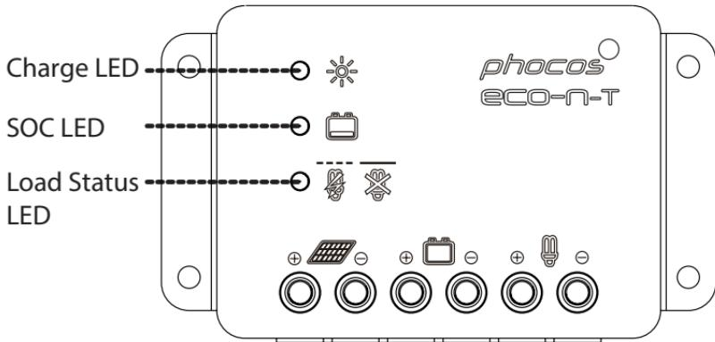
The controller is equipped with 3 LEDs to display the operating status.
