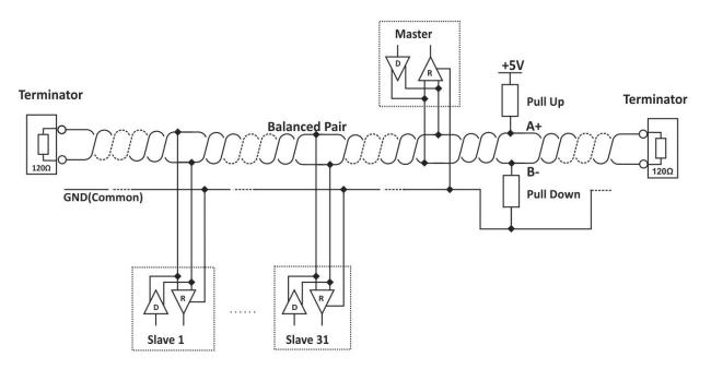
A daisy-chain (linear) topology and UTP/FTP cables for multiple sensors are strongly recommended. For proper operation of the interface, terminators (120 ohms resistors) must be installed at both ends of the bus. The device has a built-in 120-ohm resistor and to terminate the line, "Line-B-"and "Term" must be shortened.
