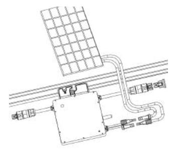
Fig.1 Installation position of microinverter
