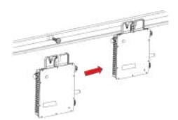
\*Note: Please install the microinverter at least 50cm above the ground/roof for better communication with Hoymiles DTU.
